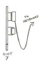
Now insert the interface card into slot # 7 of your Apple. The keyboard sits nicely either to the right or directly in front of the Apple. Your hardware should now all be connected properly. Insert your SOUNDCHASER Digital Performance Software into your Disk Drive and turn on your Apple.
