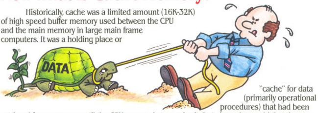
retrieved from memory until the CPU was ready to receive it. Data in cache would then be transferred to the CPU electronically where the actual processing would take place.
