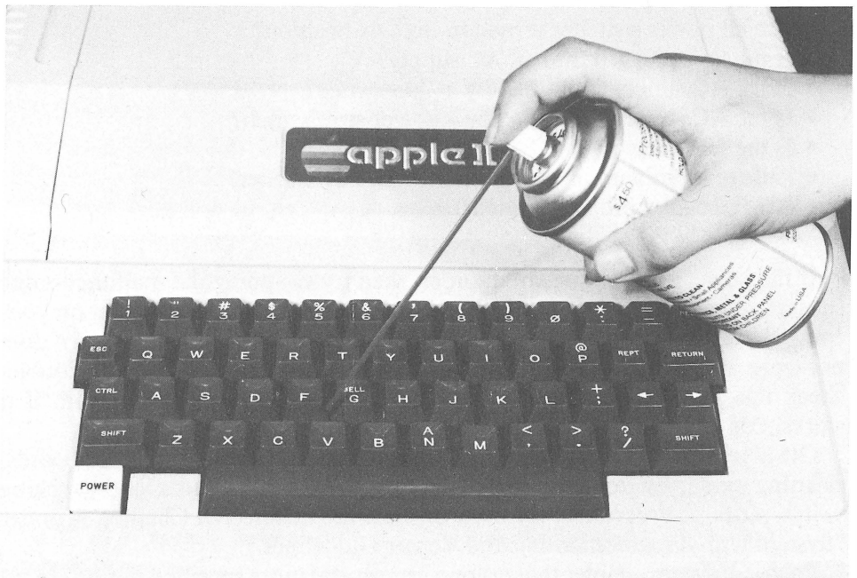
Fig. 1-4. Dusting with compressed air.
