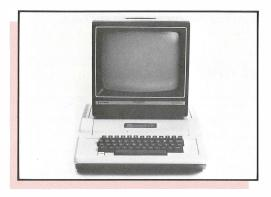
Plug one end of the video cable into the jack marked Video Out on the rear of the Apple II Plus. Plug the other end into the input jack at the back of the monitor. Plug the monitor's power cord into the wall socket.
