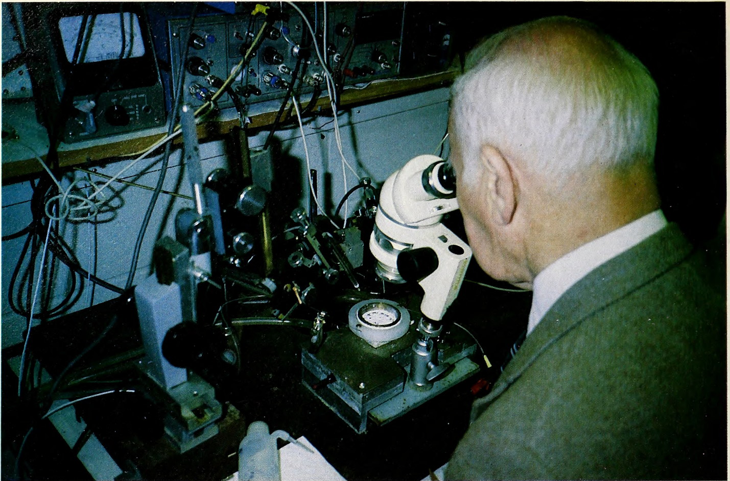
George Stibitz gazes into an electron microscope surrounded by the scope's meters and readouts. Stibitz is working on a voice board to have an Apple read the meters out loud so that the researcher can give full attention to what's happening on the other side of the eyepiece.
