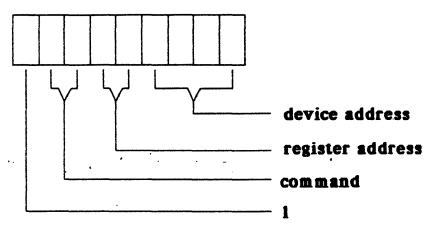
Note that the MSB of all commands is set to "1". Only the bus master has the ability to drive the MSB of any transaction on the bus to a "1". Conversely, all data transactions have the MSB set to "0". The bus master as well as any other device on the bus has the ability to set the MSB to "0".
