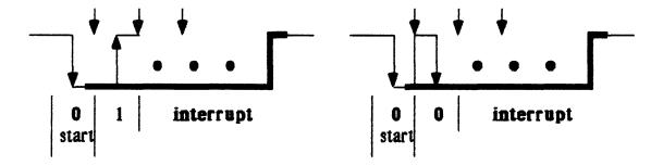
Reset has the effect that it "unlistens" all devices that have been previously addressed to LISTEN; it resets all pending interrupts; it turns the interrupt mode to DISABLE; and in general puts the devices in a mode inwhich they will accept commands. Reset issues a break on the bus by holding the bus low for a minimum of 2 ms. (This in order not to be confused with a start bit suggests that the minimum speed of the bus be a bit cell period of < 3 ms.)
